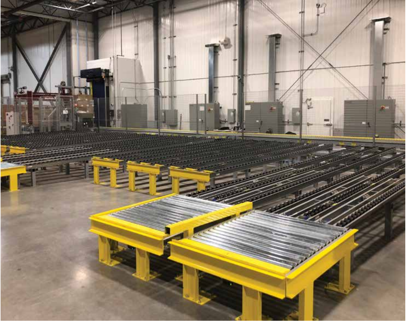
There is a pinwheel design on both inbound and outbound conveyance, which allows for efficient pallet handling in the loading and unloading processes. (Photo courtesy of UISC.)
